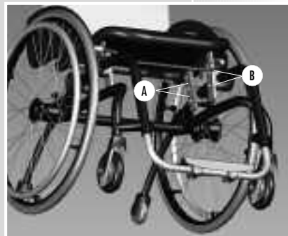
Setting the seat height, sitting angle and riding characteristics
